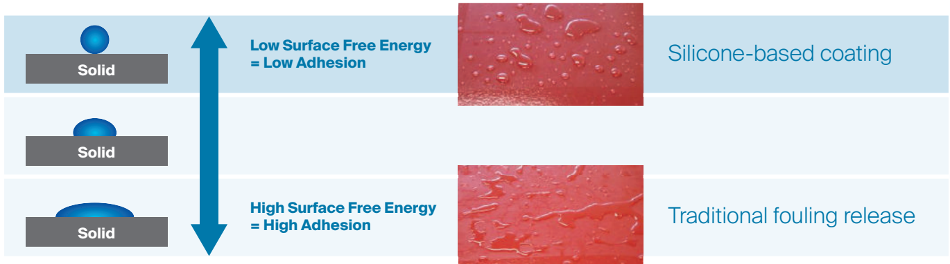
The low surface free energy of silicone-based coating
