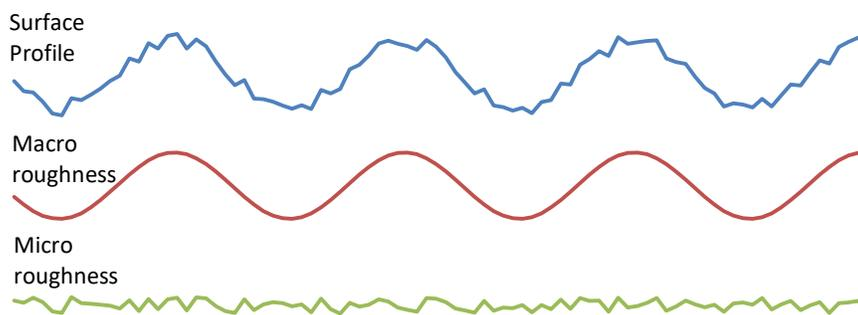
. Figure 1: A surface profile (blue) divided into macro roughness (red) and micro roughness (green).
