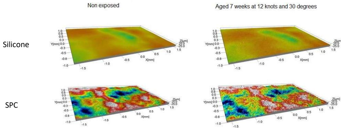
*Figure 3: Surfaces displaying micro roughness of a silicone based coating and a conventional antifouling measured by laser profilometry when freshly applied and after being exposed to sea water at 30°C for 7 weeks, at 12 knots.*
