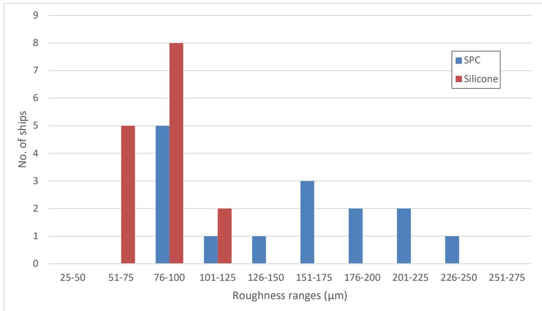
Figure 2: AHR values (µm) measured using a TQC roughness analyser on different ship types such as crude oil tankers, containers and bulk carriers and different vessel age. The measurements have been carried out for both silicone coated ships (red) and ships coated with SPC antifouling (blue). Whether the surface is full blasted or spot blasted during preparation, it is equally distributed between the ships coated with silicone or those coated with SPC.
